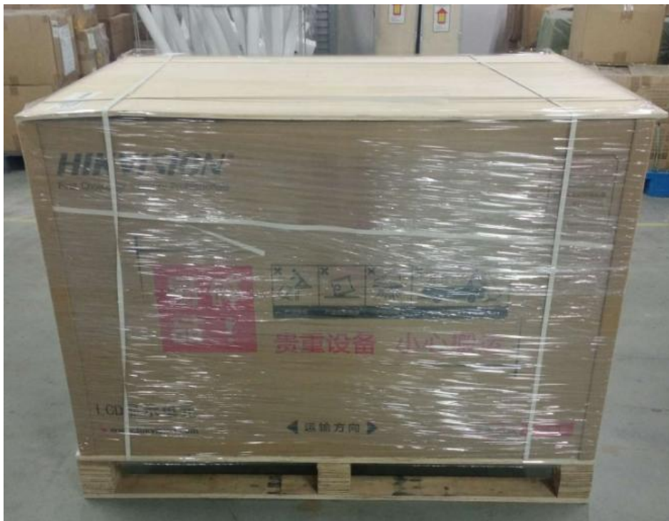
Figure 11. Four Cartons on One Wooden Pallet Secured by Films and Packing Straps
