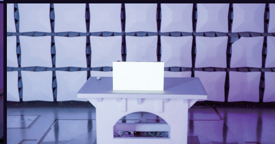
Anechoic Chamber RF Test
