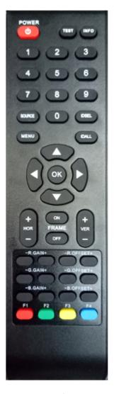
Press IDSEL to call the ID number of large screens(the original ID number of LCD unit is 0101, when delivering at porject site, different ID numbers need to be configured, the configuration can be realized with MENU)
