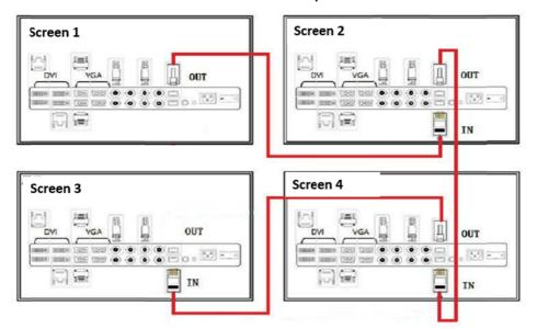
Connect the infrared probe to IR IN of Screen 1(the source of control signals), and put the other side on the front of LCD display unit, making sure the infrared signals from remote control can be detected
