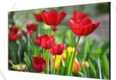
The DS-D2055UL-1B(H) LCD display uses an industry-level ultra-narrow bezel design, which enables a bezel width of 3.5 mm between neighboring displays. The adopted direct-lit LED backlighting technology helps achieve ultra-high and uniform brightness of 500 cd/m<sup>2</sup> without boundary shadows. The display has abundant interfaces for video inputs, such as DVI, VGA, HDMI, and DP.
