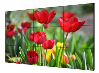
The DS-D2055UL-1B(UHK) LCD display uses an industry-level ultra-narrow bezel design, which enables a bezel width of 3.5 mm between neighboring displays. The adopted direct-lit LED backlighting technology helps achieve ultra-high and uniform brightness of 500 cd/m<sup>2</sup> without boundary shadows. The display has abundant interfaces for video inputs, such as DVI, VGA, HDMI, and DP.
