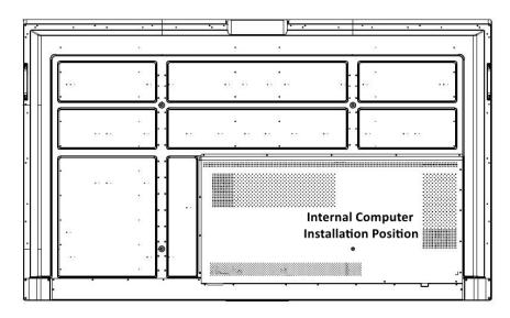
Figure 3-4 Internal Computer Installation
