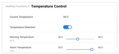
Figure 6-12 Intelligent Temperature Control
