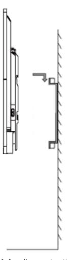
Figure 3-6 Wall Mounting Side View
