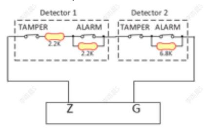
System can tell the different resistor values between Z and G for different alarms.
