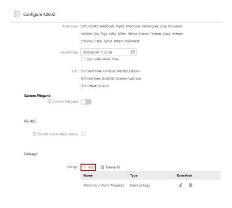
For Event type select Alarm Input Event and Alarm Input Alarm Triggered. Source Casein 01.
