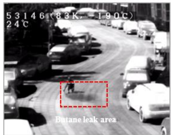
Gas Leak Detection (50 meters away, butane) Result
